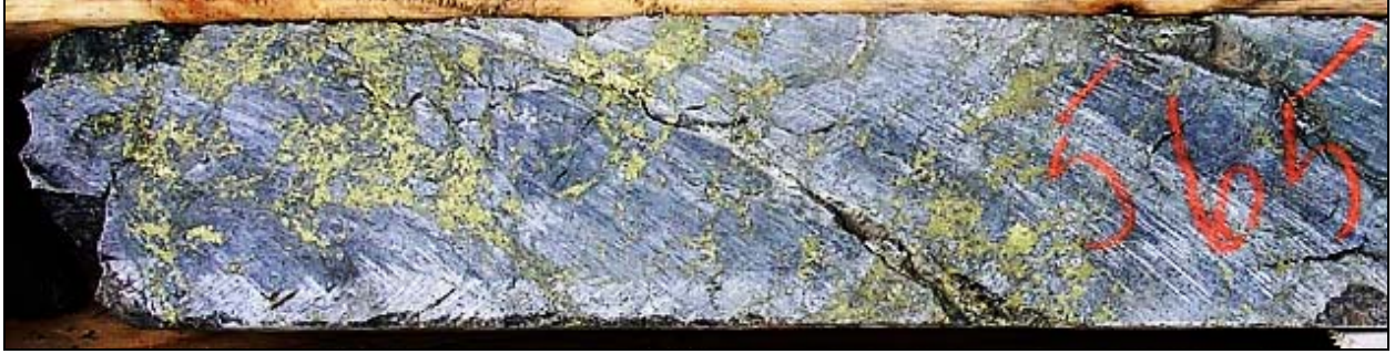
Chalcopyrite micro-veining in drill core from the Copper Prince Property.
